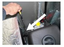
WAIT 2 MINUTES THEN REMOVE DIP STICK. (YELLOW HANDLE) WIPE OFF WITH CLEAN PAPER TOWEL. RE-INSERT DIPSTICK AND CHECK OIL LEVEL. (LOOK VERY CLOSELY OIL MAY BE VERY CLEAN AND HARD TO SEE) IF OIL IS NEEDED ADD ONLY APPROXIMATELY AN EIGHTH OF A QUART OF SYNTHITIC 10W30. WAIT 2 MINUTES TO ALLOW OIL TO DRAIN TO THE BOTTOM OF ENGINE AND CHECK AGAIN. IF MORE OIL IS NEEDED ADD
