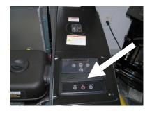
SHUT YOUR NEVER DARK GENERATOR OFF BY PRESSING THE OFF SWITCH. THIS MAY BE PUSH BUTTON OR A ROCKER SWITCH DEPENDING ON YOUR MODEL.
