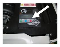
LIFT THE TOP LID OF THE GENERATOR PUSHING DOWN ON THE CORNER OF THE LID WHILE UNLOCKING (RUBBER GASKET MUST BE DEPRESSED TO EASE THE LOCKING AND UNLOCKING OF LID) SHUT GENERATOR OFF BY PRESSING THE OFF SWITCH. THIS MAY BE PUSH BUTTON OR A ROCKER SWITCH DEPENDING ON MODEL
