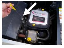
WAIT 2 MINUTES THEN REMOVE DIP STICK. WIPE OFF WITH CLEAN PAPER TOWEL. RE-INSERT DIPSTICK AND CHECK OIL LEVEL. (LOOK VERY CLOSELY OIL MAY BE VERY CLEAN AND HARD TO SEE) IF OIL IS NEEDED ADD ONLY APPROXIMATELY AN EIGHTH OF A QUART OF SYNTHITIC 10W30. WAIT 2 MINUTES TO ALLOW OIL TO DRAIN TO THE BOTTOM OF ENGINE AND CHECK AGAIN. IF MORE OIL IS NEEDED ADD ONLY APPROXIMATELY AN
