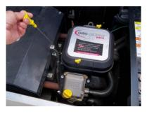
WAIT 2 MINUTES THEN REMOVE DIP STICK. WIPE OFF WITH CLEAN PAPER TOWEL. RE-INSERT DIPSTICK AND CHECK OIL LEVEL. (LOOK VERY CLOSELY OIL MAY BE VERY CLEAN AND HARD TO SEE) IF OIL IS NEEDED ADD ONLY APPROXIMATELY AN EIGHTH OF A QUART OF SYNTHITIC 10W30. WAIT 2 MINUTES TO ALLOW OIL TO DRAIN TO THE BOTTOM OF ENGINE AND CHECK AGAIN. IF MORE OIL IS NEEDED ADD ONLY
